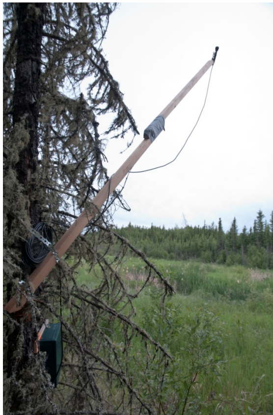
Figure 1 - Method use to set bat microphone and SM2BAT+ at edge of wetland. Note the microphone in this setup is facing up which is not optimal when raining. It is recommended by manufacturer to be parallel or slightly down relative to the ground.
